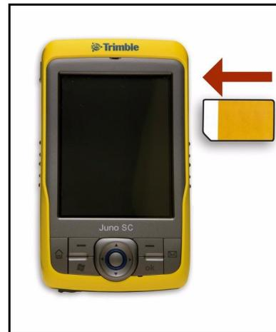
To remove the SIM card from the SIM card slot, gently press the card in and then let go. The card pops out.
