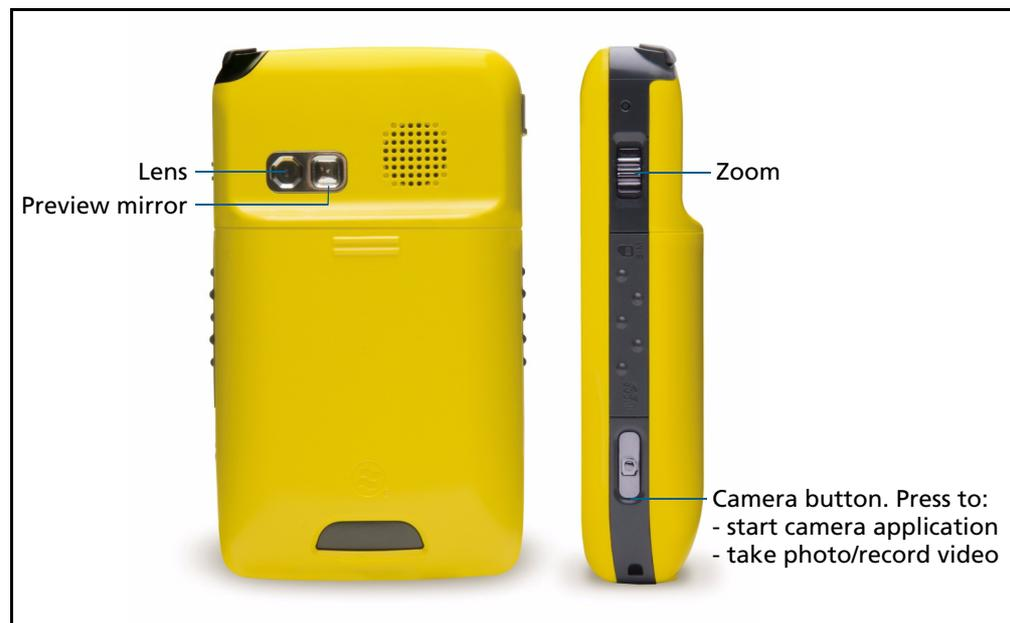
Figure 6.1 Juno series handheld – camera controls
